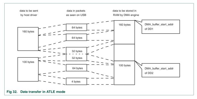
Figure 32 shows a typical OUT USB transfer in ATLE mode, where the host concatenates two USB transfers of 160 bytes and 100 bytes, respectively. Given a MaxPacketSize of 64, the device hardware interprets this USB transfer as four packets of 64 bytes and a short packet of 4 bytes. The third and fourth packets are concatenated. Note that in Normal mode, the USB transfer would be interpreted as packets of 64, 64, 32, and 64 and 36 bytes.
