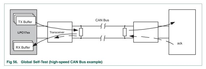
Initiating a Global Self-Test is similar to a normal CAN transmission. In this case the transmission of a CAN message(s) is initiated by setting Self Reception Request bit (SRR) in conjunction with the selected Message Buffer bits (STB3, STB2, STB1) in the CAN Controller Command register (CANCMR).
