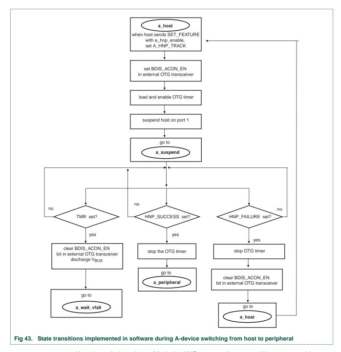
Note that only the subset of A-device HNP states and state transitions supported by hardware are shown. Software is responsible for implementing all of the HNP states.
