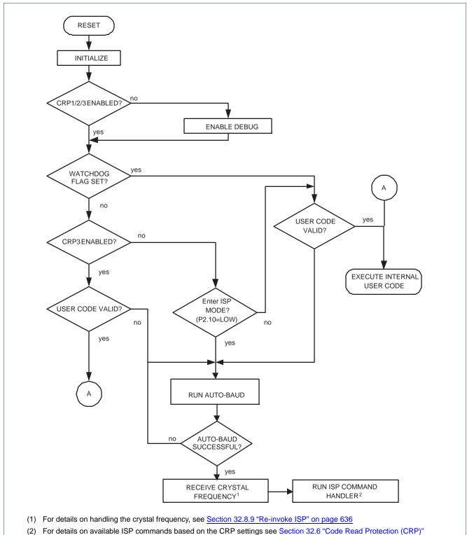
Fig 137. Boot process flowchart
