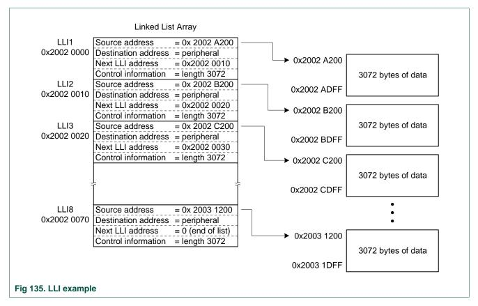
The first LLI, stored at 0x2002 0000, defines the first block of data to be transferred, which is the data stored from address 0x2002 A200 to 0x2002 ADFF:
