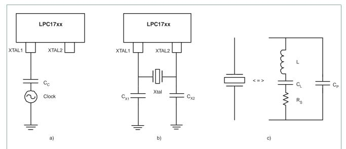
Fig 8. Oscillator modes and models: a) slave mode of operation, b) oscillation mode of operation, c) external crystal model used for  $C_{X1}/X_2$  evaluation
