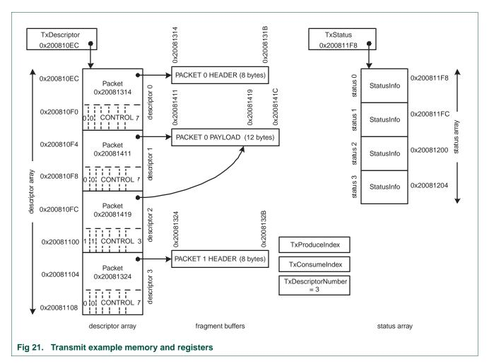
After reset the values of the DMA registers will be zero. During initialization the device driver will allocate the descriptor and status array in memory. In this example, an array of four descriptors is allocated; the array is 4x2x4 bytes and aligned on a 4 byte address
