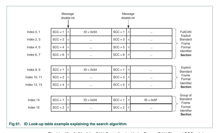
The identifier 0x5A of the CAN Controller 1 with the Source CAN Channel SCC = 1, is defined in all three sections. With this configuration incoming CAN messages on CAN Controller 1 with a 0x5A identifier will find a match in the FullCAN section.
