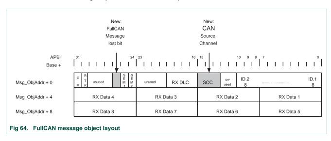
The new message lost bit (MsgLst) is introduced to indicate whether more than one FullCAN message has been received since last time this message object was read. For more information the CAN Source Channel (SCC) of the received FullCAN message is added to Message Object.
