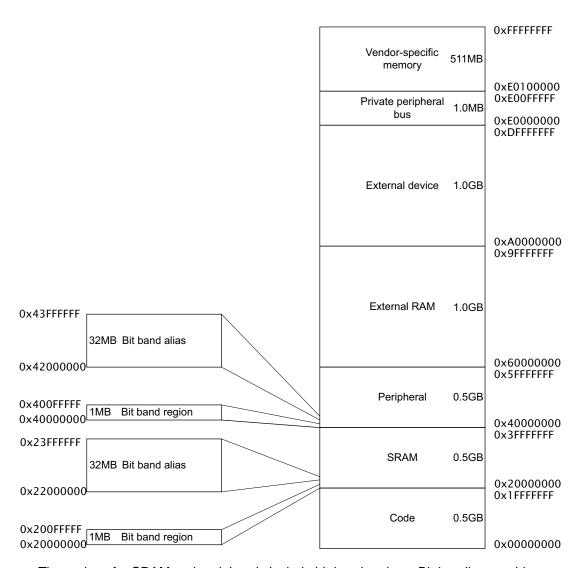
The regions for SRAM and peripherals include bit-band regions. Bit-banding provides atomic operations to bit data, see <a href="Section 34.3.2.5">Section 34.3.2.5</a>.
