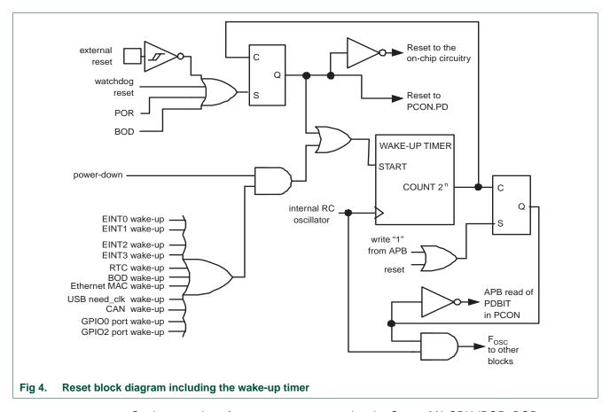
On the assertion of a reset source external to the Cortex-M3 CPU (POR, BOD reset, External reset, and Watchdog reset), the IRC starts up. After the IRC-start-up time (maximum of 60  $\mu$ s on power-up) and after the IRC provides a stable clock output, the reset signal is latched and synchronized on the IRC clock. Then the following two sequences start simultaneously:
