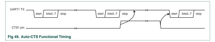
While starting transmission of the initial character the CTS1 signal is asserted. Transmission will stall as soon as the pending transmission has completed. The UART will continue transmitting a 1 bit as long as CTS1 is de-asserted (high). As soon as CTS1 gets de-asserted transmission resumes and a start bit is sent followed by the data bits of the next character.
