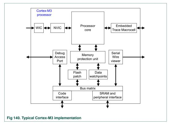
The Cortex-M3 processor is built on a high-performance processor core, with a 3-stage pipeline Harvard architecture, making it ideal for demanding embedded applications. The processor delivers exceptional power efficiency through an efficient instruction set and extensively optimized design, providing high-end processing hardware including single-cycle 32x32 multiplication and dedicated hardware division.
