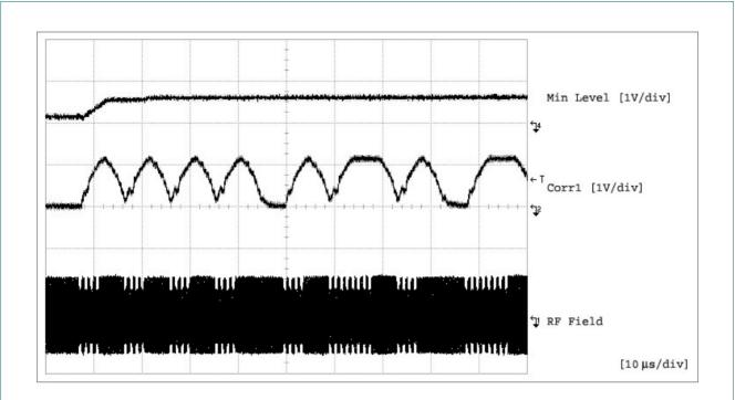
Fig 25. Output Testsignal Corr1 on AUX1 and MinLevel on AUX2.
