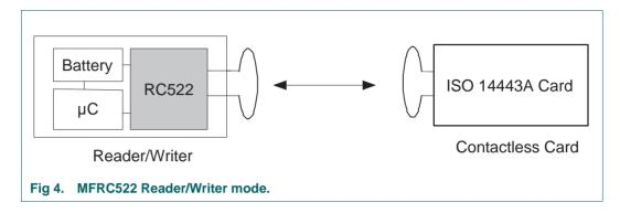
The following diagram Figure 5 "ISO/IEC 14443A/MIFARE® Reader/Writer mode communication diagram." describes the communication on a physical level.
